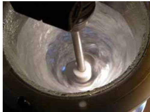
Counter flow impeller at work
